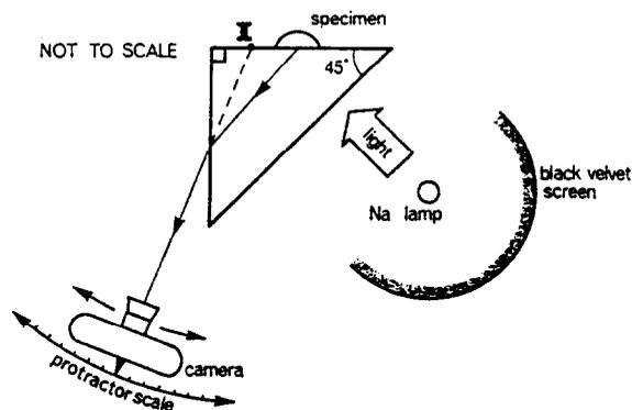
FIG. 2. Pulfrich refractometer adapted to photograph lens sections with sodium light. The camera arm is pivoted about the image I of the specimen.
