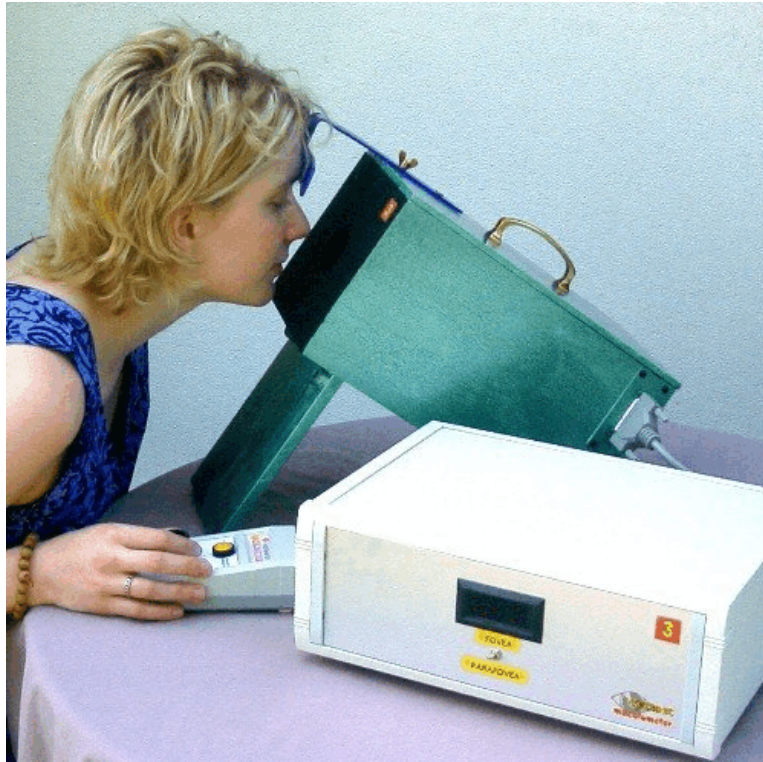
Figure 6 A screening maculometer (Mellerio et al. 2002)
